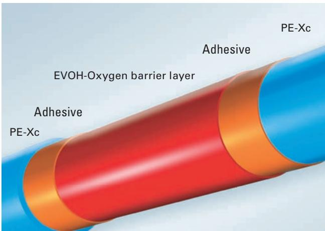
Using a new developed extrusion procedure, Hewing can process five layers into a homogenous pipe in a single production step. Following subsequent final cross-linking, the pipe is finished: the Penta-Pipe, featuring a centrally positioned oxygen barrier layer. It is equipped with a particularly robust PE-Xc outer pipe, securely connected to the oxygen barrier via a further adhesive layer. Thus, Penta-Pipe is protected from damage on construction sites as well as in operation.
